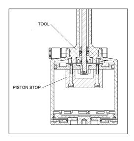
Regular servicing should be carried out and a comprehensive inspection performed annually or every 500,000 cycles, whichever is sooner.
